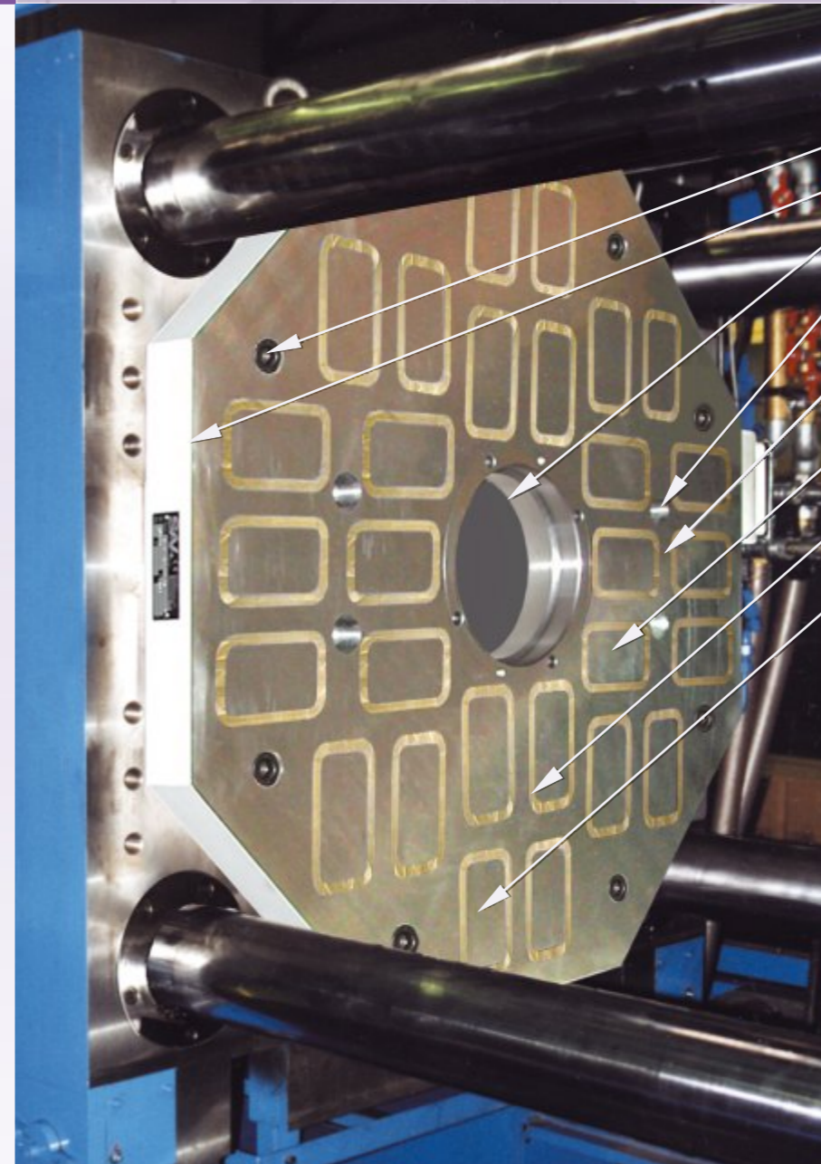
EP-QMC magnet on a 15 ton machine. With rolling system for tool change, including sliding table and preheating station. Drastic reduction of machine downtime due to preheating parallel to operation.
