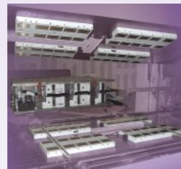
High energy Electro permanent magnets for clamping of deep pulling tools, workpiece weight 8 ton. Including hydraulic rolling system for tool change.
